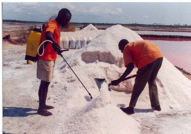
Figure 2 Iodation of salt using a knapsack sprayer and manual mixing of a 2-ton salt heap.
