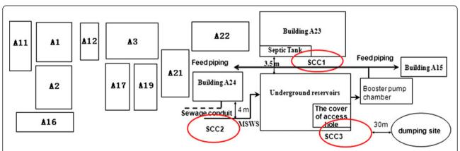
**Figure 1 Schematic of environment around underground reservoirs in the factory having gastroenteritis outbreak.** SCC1: the first suspected source of contamination. SCC2: the second suspected source of contamination. SCC3: the third suspected source of contamination. MSWS: Municipal supply water system. Building A1, A3, A11, A12, A15, A21, A22, A23 provide DDWD. Building A2, A16, A17, A19 provide bottled water.
