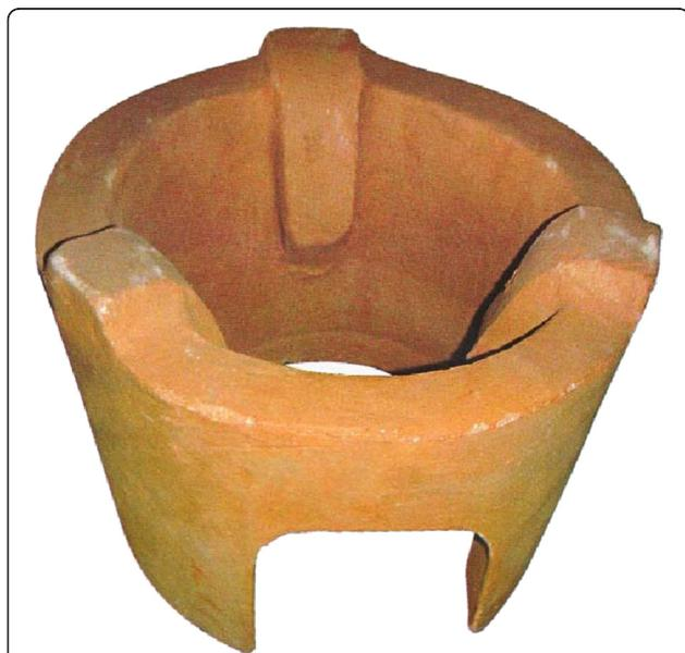
**Figure 1** *Upeski jiko* (ceramic-lined cookstoves), Nyanza Province, Kenya<sup>a</sup>. <sup>a</sup> The specific dimensions of the stove are 26 centimeters diameter for the internal bottom, 30 centimeters for the internal diameter, 15 centimeters curved for the door size, 1 centimeter for the height of the pot rest, and 18 centimeters for the height of the firebox.
