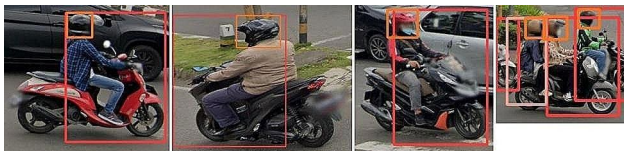
Fig. 2 Labeled images with manually drawn bounding boxes around object classes
