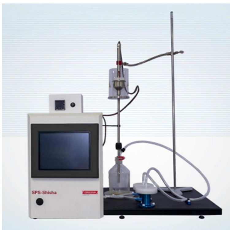
Fig. 1 Laboratory water-pipe equipment (SPS SHISHA—Specialist shisha pipe smoking machine) complying with ISO 22486:2019 and used according to method ISO/TS 22487:2019
