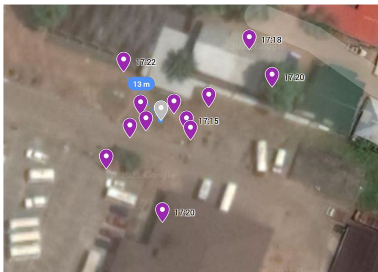
Fig. 2 Measurement of accuracy during use in an outside urban environment. Distance of logged GPS coordinate (violet) to location of the participant (grey) in m. Time of logged GPS coordinate in hh:mm
