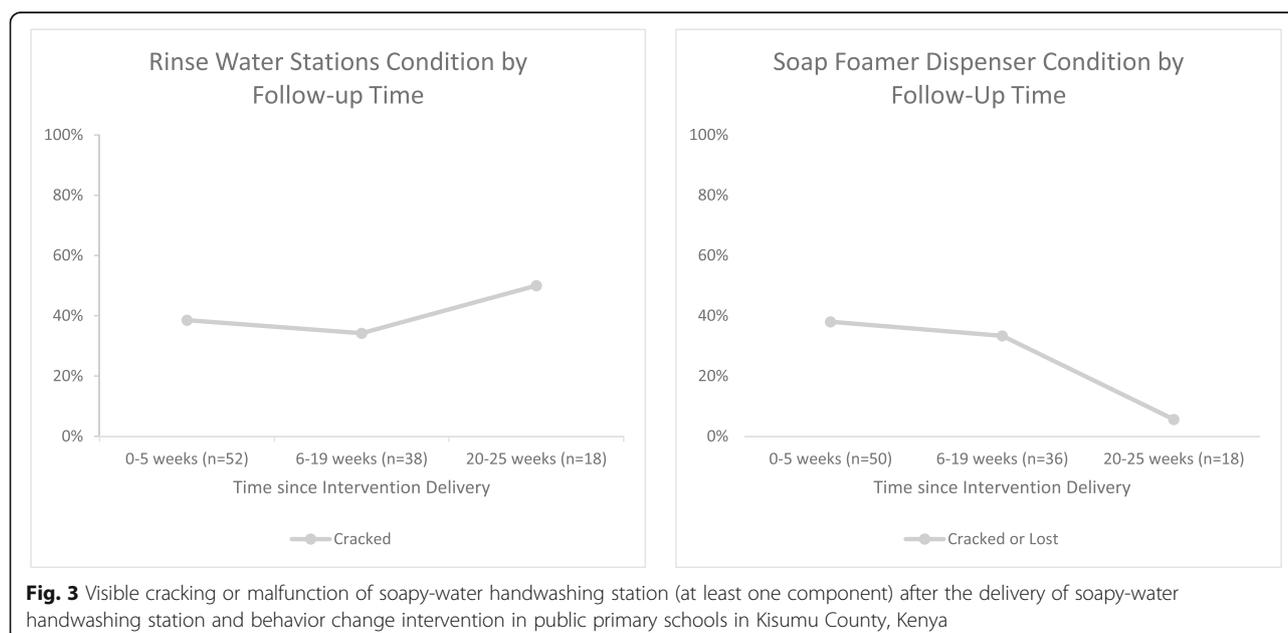
**Fig. 3** Visible cracking or malfunction of soapy-water handwashing station (at least one component) after the delivery of soapy-water handwashing station and behavior change intervention in public primary schools in Kisumu County, Kenya
